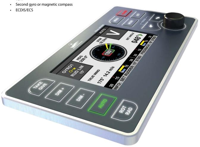
Three more control modes have been added to those present in the previous generation of the AP4000: the 'CTS Pilot' control mode, which allows for steering by a pre-set COG value, the 'Windvane' mode for sailing yachts, making it possible to steer by setting the relative wind angle, and the 'River Pilot' mode, allowing the operator to steer the vessel by a pre-set ROT value using an external ROT tiller or the knob in the control panel.
