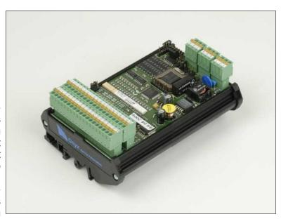
a series of input diodes that avoids current returns when the module is switched off, it allows the parallel connection of inputs to discrete backup circuits for alarm detection.
