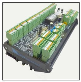
The OM-961S module is a slave unit, and it is used to handle the switchover between primary and secondary CANbus paths at board or switchboard level.
