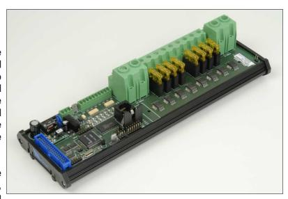
modes (breaker, cabin lights, bilge pump, timer-controlled tank pump and navigation lights) of each channel can be configured. The configuration can be done by the CAN network or locally, thanks to the optional programming keyboard. In case of fault of the electronic, a bypass cable (available as option), fuse protected, can be used to activate each output.
