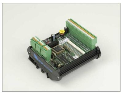
environment: the use of extended temperature range components (-20 to +85 °C) and Type Approval certification make it an invaluable element for a modern marine automation system.
